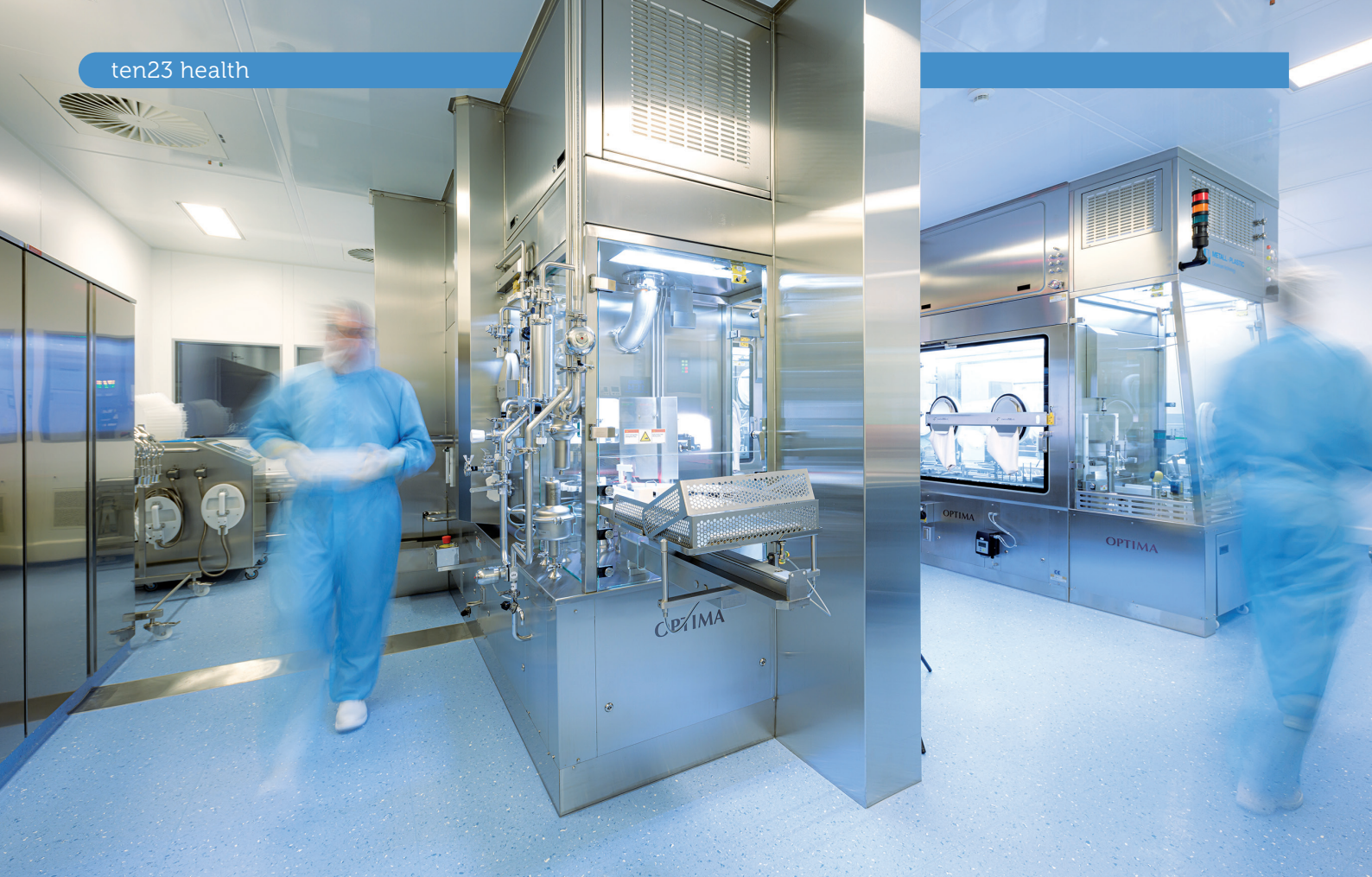
Figure 2: ten23's facilities include the capability for highly accurate, air-bubble-free filling of very low-volume primary containers in isolators operated in class C.
